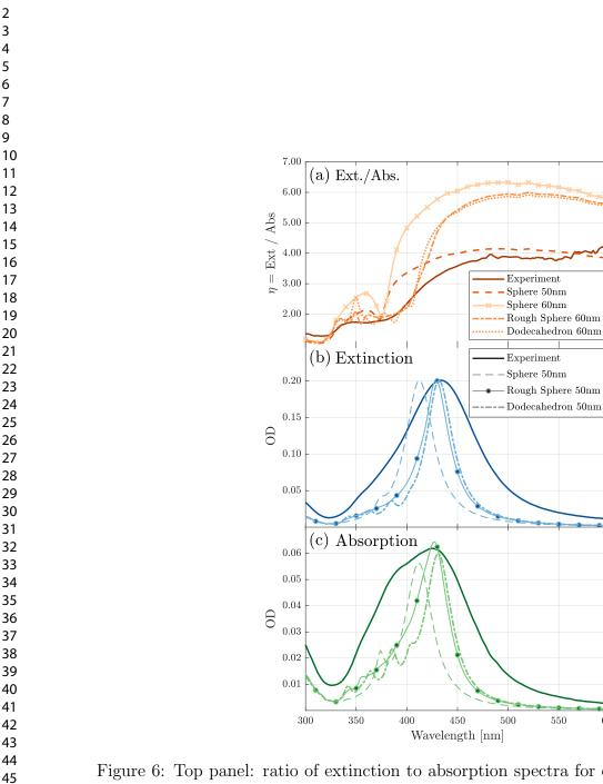
Figure 6: Top panel: ratio of extinction to absorption spectra for our measured NPs (solid line) along with a number of representative predictions: 50 and 60 nm spheres, a 60 nm roughened sphere ( $\delta r = 1.4$  nm) and a dodecahedron (radius of the equivalent-volume sphere: 60 nm). Middle and bottom panels: Extinction and absorption spectra for a 50 nm sphere, a rough sphere ( $\delta r = 1.4$  nm) and a dodecahedron compared to experiments (solid lines).
