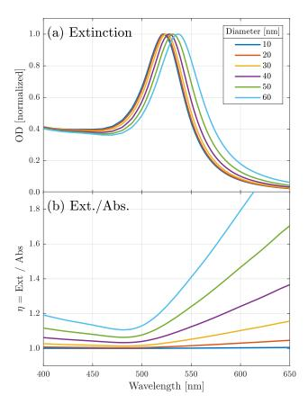
Figure 7: Predicted extinction spectra (a) and extinction to absorption ratios (b) for gold nanospheres of varying diameter in water, calculated using Mie theory and the gold dielectric function from Ref.<sup>60</sup>
