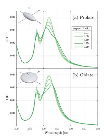
Figure 3: Absorption spectra of prolate (top panel) and oblate (bottom panel) silver NPs of different aspect ratio in water, calculated using the *T*-Matrix method.
