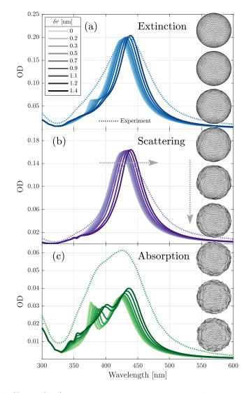
Figure 5: Predicted (from SIE) extinction, scattering and absorption spectra of spherical silver NPs of different rms roughness  $\delta r$ . The NPs are in water and have the same volume as a 60 nm sphere. In each panel, the experimental spectrum is plotted in dotted lines.
