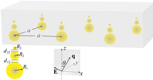
Fig. 1. (Color online) Schematic view of a square lattice of nanolenses in a glass matrix. Each nanolens consists of three silver spheres with decreasing radii  $R_1 = 33.8$  nm,  $R_2 = 13$  nm, and  $R_3 = 5$  nm, and separations  $d_{12} = 7.8$  nm and  $d_{23} = 3$  nm.
