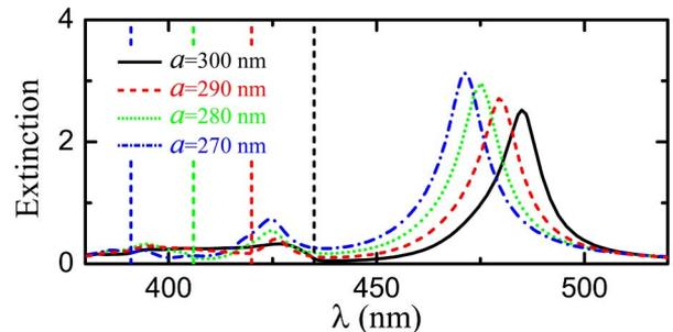
Fig. 3. (Color online) Extinction spectra of square arrays of the nanolens motif under consideration in a glass matrix, for  $p$ -polarized light incident at an angle  $\theta = 45^\circ$ , for lattice constants  $a$  varying from 270 to 300 nm. The vertical dashed lines indicate the position of RW2 in each case.
